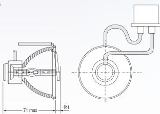
Lamp aligned for maximum throughput thru 6mm aperture at 52mm distance from reflector rim.
